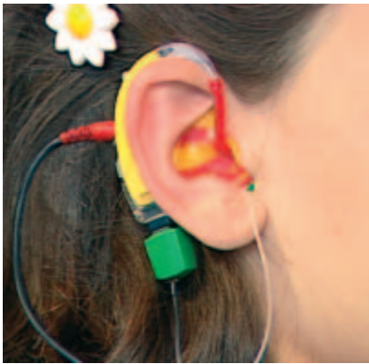
Figure 5 RECDdirect measurement setup
