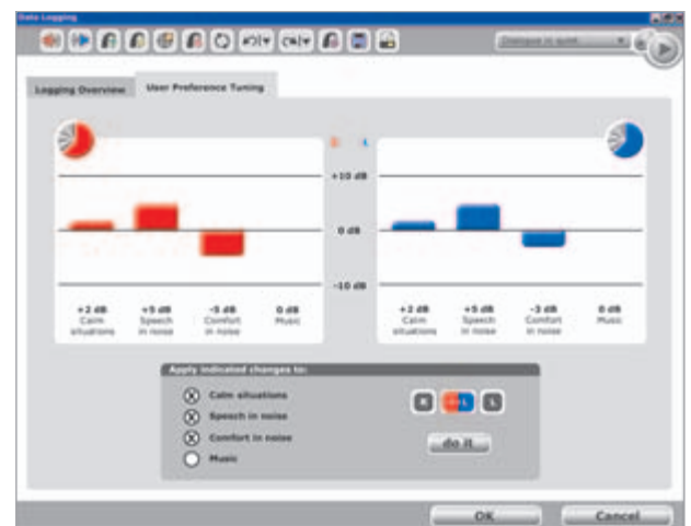
Figure 14: User Preference Tuning. Fine tuning suggestion based on actual volume changes done by the client in daily life.
