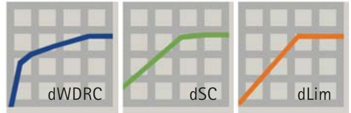
Fig. 1: Typical input/output transfer functions for WDRC, SC and linear processing.
