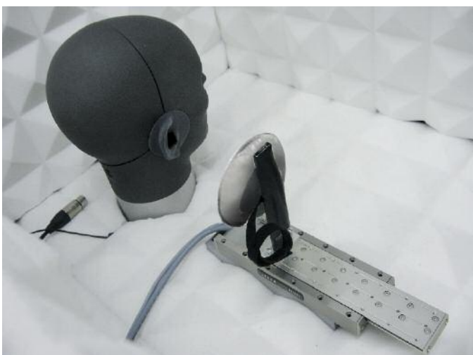
Figure 3: Test set-up for assessing the performance of feedback management systems under reproducible conditions.
