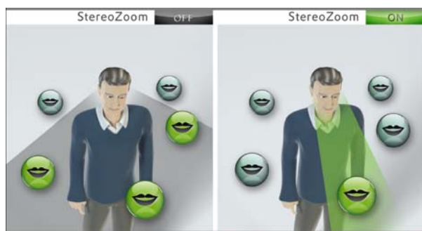
Fig. 6: Monaural directional microphones have a broad forward focus (grey beam) StereoZoom creates a highly focused beam (green) to the front to focus on a single voice in a crowd.
