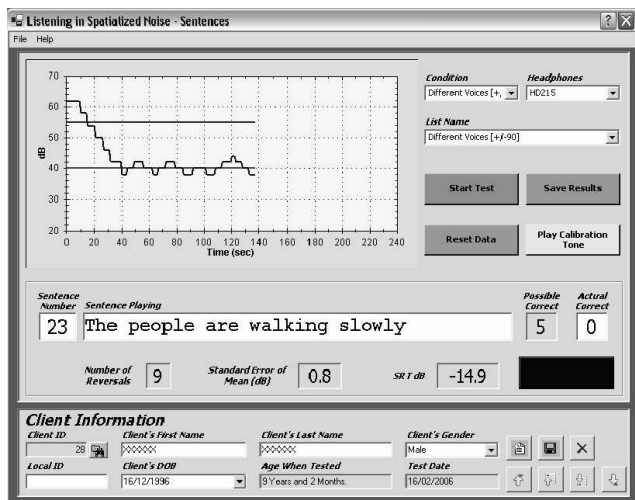
Figure 1. The LISN-S Playback Screen. The graph shows the history of the target level as the range of correct responses from >50% correct to <50% correct is repeatedly traversed. The top horizontal line shows the level of the distracters, and the lower horizontal line shows the average level of the targets during the stable region.
