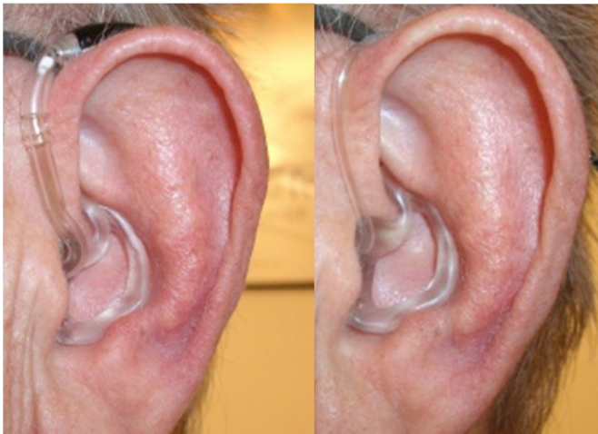
Pic. 1: Naída S with standard tube Pic.2: Naída S with Power SlimTube
