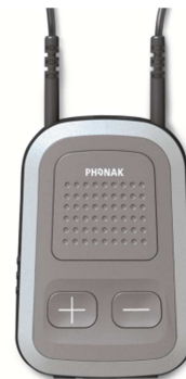
Figure 2: Phonak ComPilot manual controls
