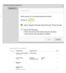
Adjustments and modifications to the programs can be made in [Fine tuning]. Click [All programs] to adjust all programs simultaneously. Click [SoundFlow] to modify all acoustic automatic programs. To modify a single program, click on one program in the list and adjust as needed.
