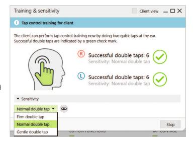
The default setting for sensitivity is "Normal". The setting "Firm" means a strong double tap motion is needed to activate Tap Control. The setting "Gentle" means a light double tap motion is sufficient to activate Tap Control.
