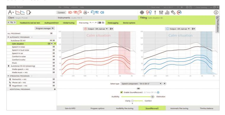
SoundRecover2 is a frequency compression system with adaptive behavior.
