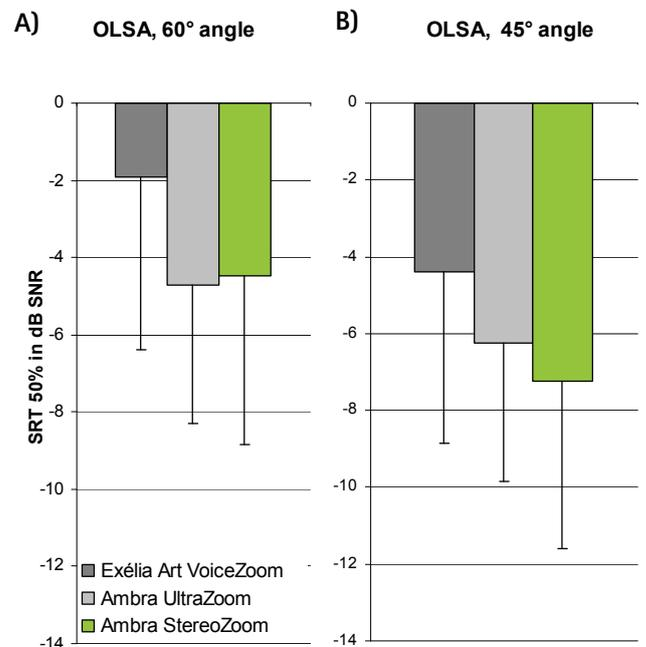
Fig. 2: Speech intelligibility scores in dB SNR of the beamformers of Exélia Art and Phonak Ambra in the OLSA, tested with two different angles to the front ( $60^\circ$  and  $45^\circ$ ). Results show clear benefits of StereoZoom for a narrower angle of  $45^\circ$  to the front, thereby focusing on a single signal presentation as illustrated in Fig. 1.
