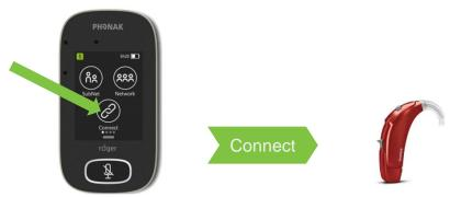
To connect, the receiver must be powered on and within 10cm/4inches of the transmitter. Tap [Connect] on the Roger Touchscreen Mic or press [Connect] on the Roger Pen, Roger EasyPen or Roger Clip-On Mic.
