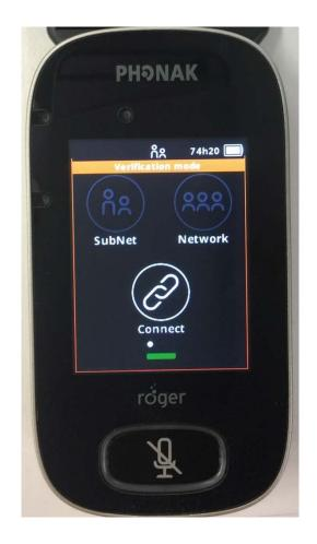
Once the Roger POP is complete, switching the respective microphone off and on again will deactivate **Verification mode** and return the microphone to standard operation.
