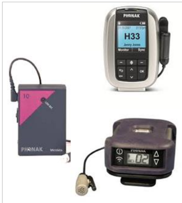
Figure 1. Examples of remote microphone systems that were worn by teachers to transmit their voice to children with hearing loss.
