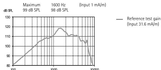
Note: Using pure tone measurements with a digital hearing instrument can result in a wavy frequency response. This is an artifact resulting from the use of a narrowband input signal and does not affect the actual performance with naturally occurring broadband input signals.
