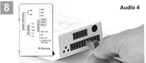
Terminate the 2-pin Phoenix connector to the CH4+/CH4- (Bal) series-socket as depicted above.
