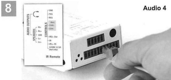
Terminate the 2-pin Phoenix connector to the CH4+/CH4- (Bal) series-socket as depicted above.
