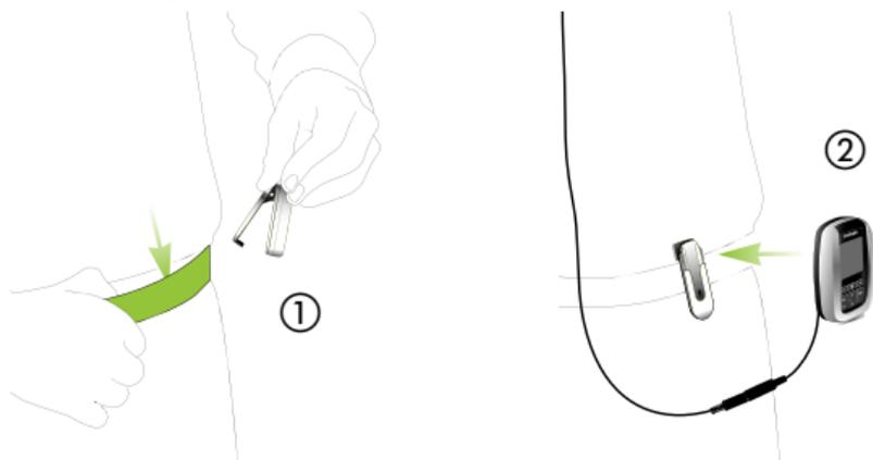
The clip can also be fixed to the belt or trousers *before* the inspiro is attached. Make sure the clip is secure.
