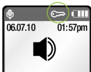
**⚠** If the key pad lock is activated, the front keys are locked. These remain locked when using the ON/OFF slider. Please note that the ON/OFF slider is never locked and can always be used!
