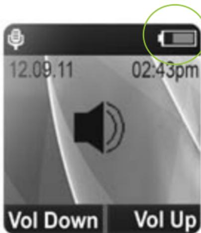
If the charging unit is removed from the inspiro, the battery symbol shows the actual capacity.
