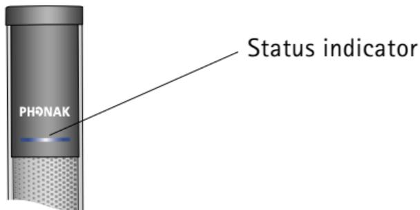
The status indicator on the DigiMaster loudspeaker provides immediate feedback to the user.
