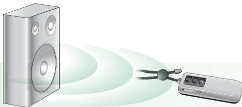
If the audio equipment does not have a headphone output socket, place ZoomLink in front of the loudspeaker of the television or the radio receiver. Then switch on ZoomLink and the television.
