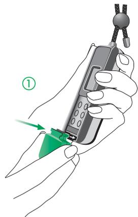
Attach the adapter to ZoomLink, then plug the MicroBoom cable into the microphone socket of the adapter.
