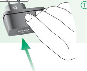
Attach the ZoomLink adapter for external connections
