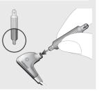
3. Do not overtwist the tool; stop when you feel a slight resistance (about 1 rotation) or you could damage the audio filter.
