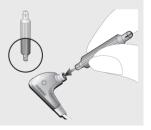
3. Do not overtwist the tool; stop when you feel a slight resistance (about 1 rotation) or you could damage the audio filter.
