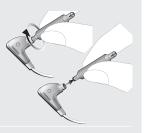
4. So you can reuse the audio filter, insert it in an empty slot in the audio filter box; turn and remove the changing tool. Dispose of any soiled or damaged audio filters.
