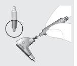
Do not overtwist the tool; stop when you feel a slight resistance (about 1 rotation) or you could damage the audiofilter. Pull the used audio filter out.
