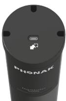
The Roger DigiMaster firmware can be upgraded over time whenever new features are available through the USB connector.
