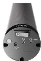
A Bluetooth connectivity module added inside the Roger DigiMaster N2 loudspeaker supports wireless connection to devices such as tablet or computer.
