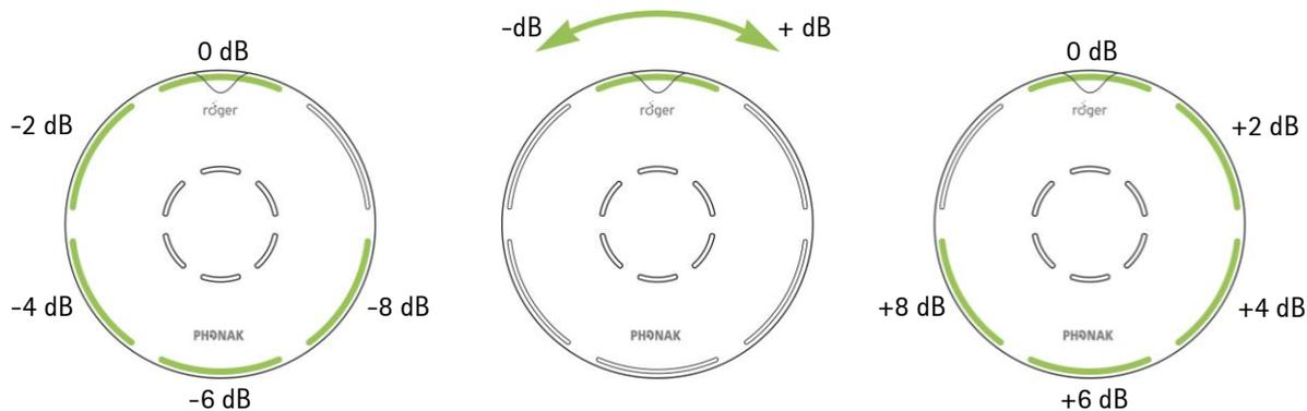
To store the new volume and end the process, tap the center touch key on Roger Select. Repeat the verification and default volume adjustment on the second receiver, if needed.
