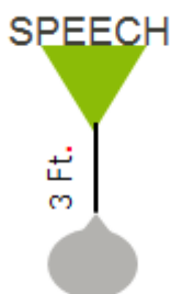
Figure 6. Schematic of the soft speech setup for comparison of speech recognition performance using automatic classification systems from three manufacturers.
