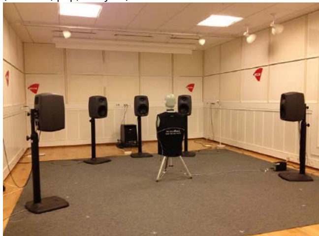
Figure 2. The setup in DELTA's EBU 3276 standardized listening room for the hearing aid recordings.
