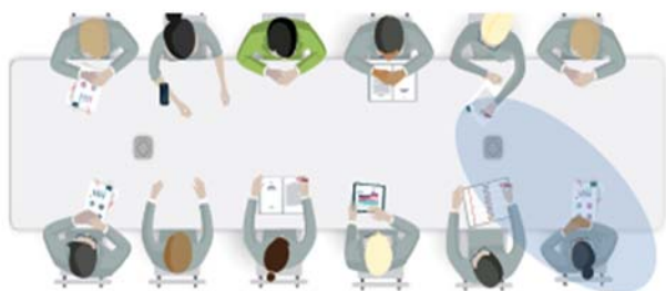
Figure 5b: Diagram illustrating a large meeting with a Table Mic II placed at each end of the conference table. Multibeam Technology selects and activates a single beam with the best SNR, shown in blue. The listener is shown in green.
