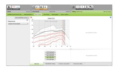
In [Basic Tuning] the [Gain level] adjustments of the hearing instrument in a BiCROS fitting will optimize the correct amplification of the hearing instrument when streaming. Changes will only apply to the hearing instrument.
