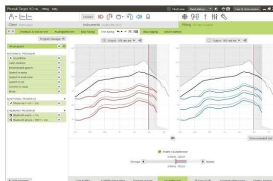
The SoundRecover fitting tool can be extended to adjust independently the cut-off frequency and the compression ratio. Click [Show extended tool] to do this.
