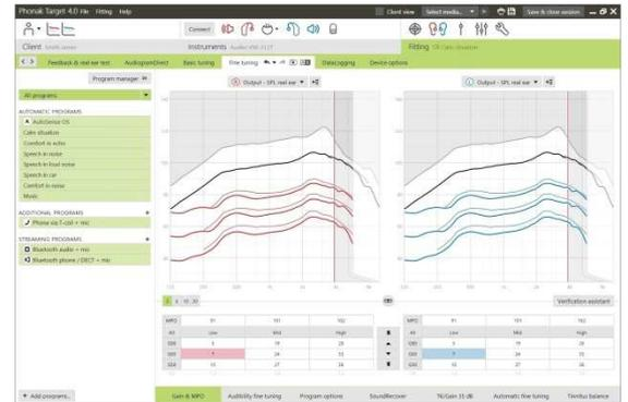
The tabs in the lower part of the screen will offer you access to the fitting tools. Each tool offers specific modifiers to fine-tune the hearing instrument
