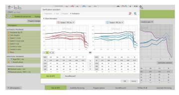
When an instrument is muted or unmuted, a watermark can be seen above the curve display (i.e. Muted or Speech). The speech watermark serves as a reminder of the recommended input signal to optimize target matching.
