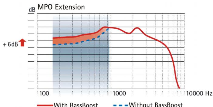
**Fig. 1:** Range and amount of MPO extension of BassBoost set to level 2 (+6dB) in a power (411) BTE instrument.
