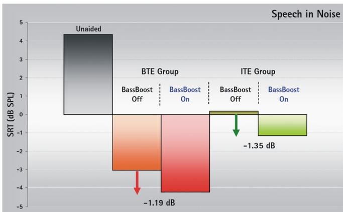
**Fig. 3:** Results from the OLSA test. BTE results with directional microphone (red) and ITE results (green).
