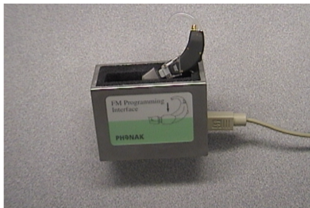
Figure 10. The Phonak Toaster allows for programming the level of the FM signal and setting the default channel of the FM Receiver.
