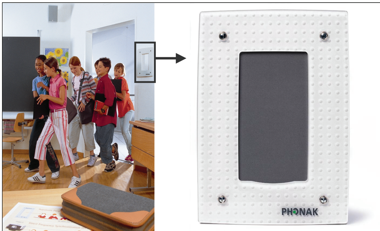
Figure 4. One type of Wireless Frequency Selection (WFS) is Automatic Frequency Synchronization (AFS) which causes the FM Receiver to automatically change to the set channel when the student walks within three feet of the wall panel shown on the left. The wall panel is shown on the right. Photos courtesy of Phonak Hearing Systems.
