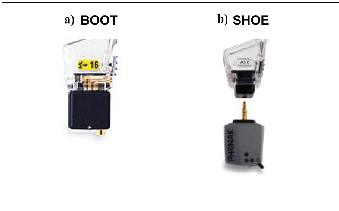
Figure 5. Suggested use of the labels a) “boot” and b) “shoe.” The single-component arrangement where the FM Receiver is hard-wired to the component that fits on the base of the BTE could be referred to as the “boot” and the two-component system where the FM Receiver attaches to the component that then attaches to the base of the BTE aid could be referred to as the “shoe.” Photos courtesy of Phonak Hearing Systems.
