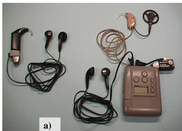
Figure 10. The Phonak Toaster allows for programming the level of the FM signal and setting the default channel of the FM Receiver.
