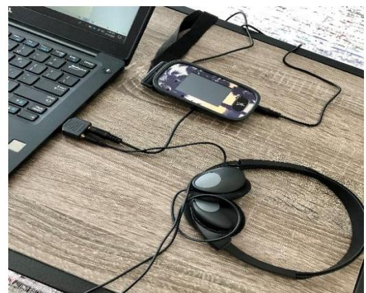
Here is a high-level overview of how to connect DM/FM/Streaming devices through a splitter to a student's computer or tablet.
