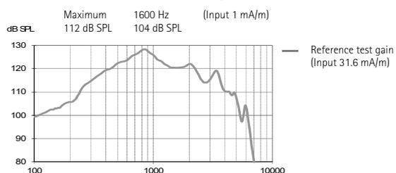
Using pure tone measurements with a digital hearing instrument can result in a wavy frequency response. This is an artifact resulting from the use of a narrowband input signal and does not affect the actual performance with naturally occurring broadband input signals.
