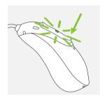
If the hearing aid is paired with a Bluetooth® enabled phone, a short press on the upper or the lower part of the button will accept an incoming call and a long press will reject an incoming call – refer to chapter 13.
