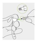
Rotate the changing tool clock-wise until some resistance is felt.
