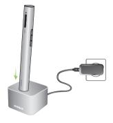
An empty battery will reach its maximum charge in approximately 2 hours. Charging is complete when the indicator light turns solid green.
